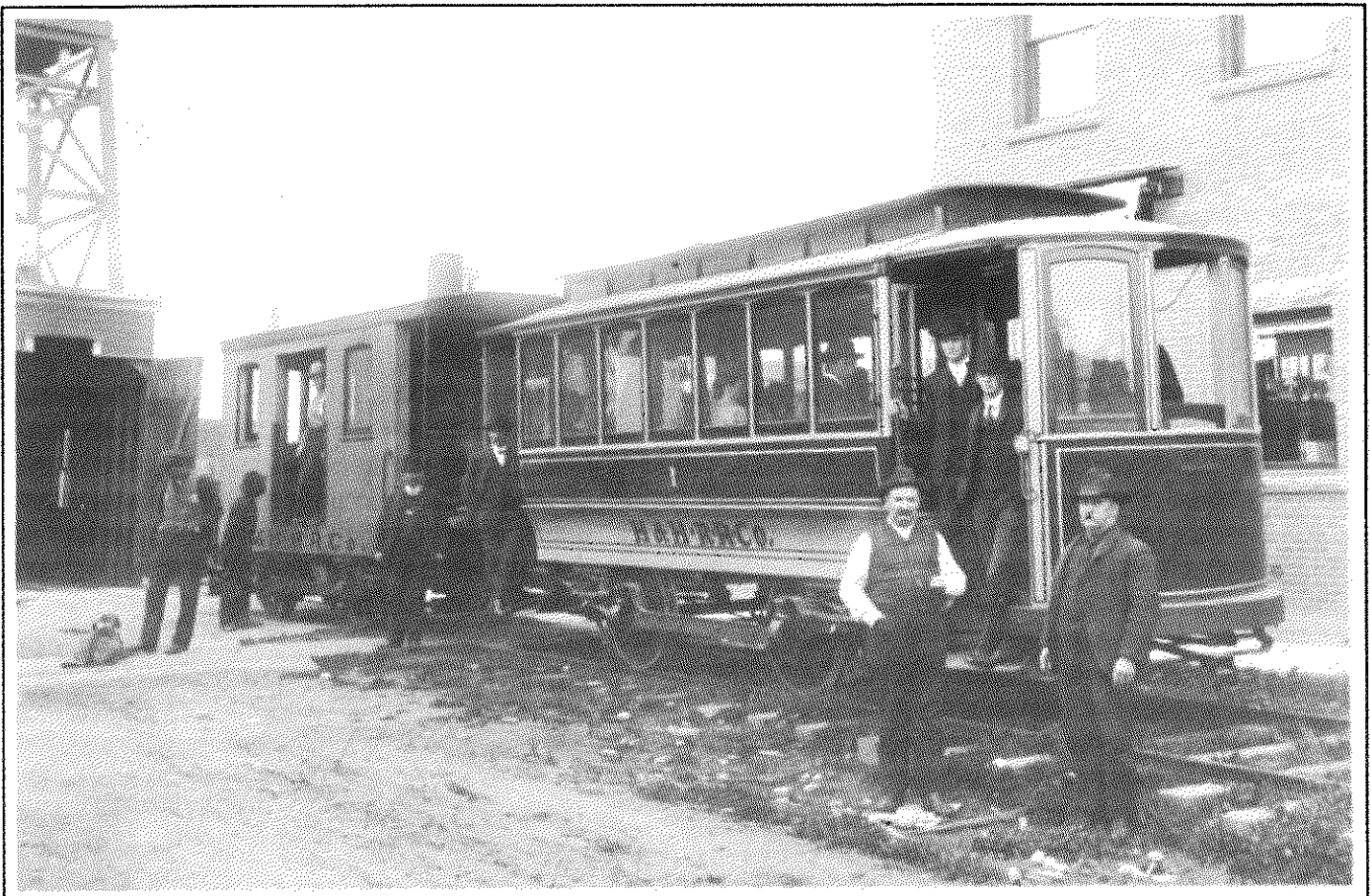
HALL & HALL RAILROAD – THE SHORTEST PRIVATELY HELD RAILROAD IN THE WORLD presumably with proud sponsors and owners standing by. This is the first version: the gasoline motor engine made in Everett and the street car from the Seattle street car line.
